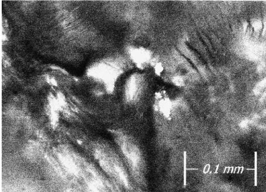
Fig. 10. SEM of the creep fracture surface of adhesively bonded joint, showing craze formation in the adhesive.
