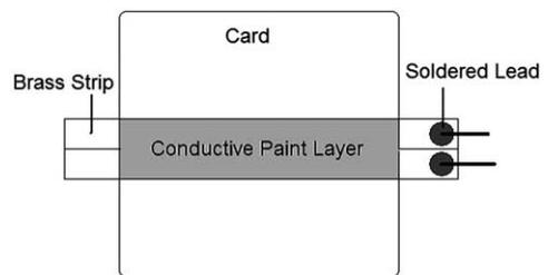
Fig. 2. Calibration sample.
