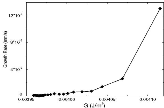
Fig. 9. Crack growth rate for steel–steel adhesively bonded specimen.
