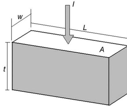
Fig. 1. Resistive element.
