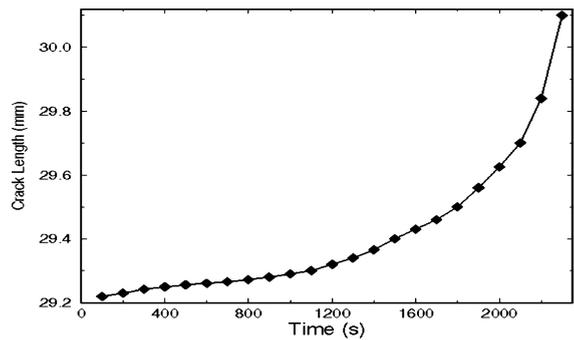
Fig. 8. Results of creep testing for steel–steel specimen.
