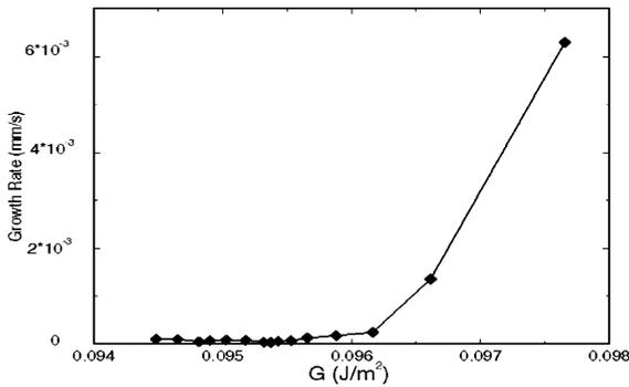
Fig. 7. Crack growth rate for brass–brass specimen.
