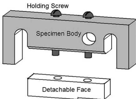
Fig. 4. Split half of the modified CTT specimen.
