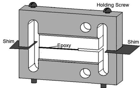
Fig. 5. Assembly of adhesive CTT specimen.
