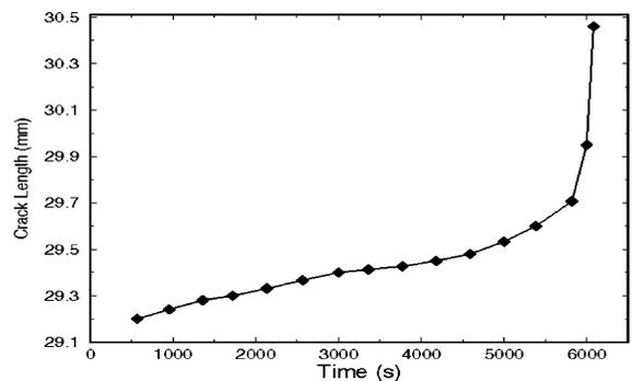
Fig. 6. Results of creep testing for brass–brass specimen.
