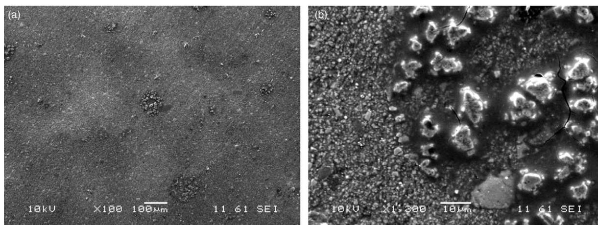
**Figure 7** (a) SEM evaluation of the particle-reinforced wear surface reveals several silica particle ‘clusters’ distributed throughout the material. (b) Examination of the ‘cluster’ at an increased magnification reveals the incidence of micro-cracking around the edges of the particles.
