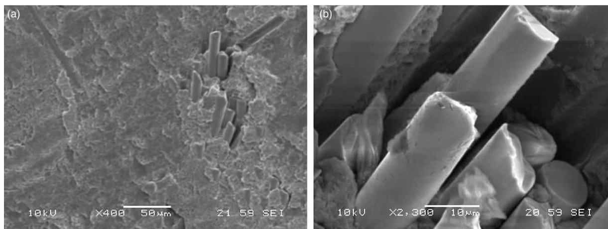
**Figure 6** The SEM photographs of the 7.6 wt% wear surface display (a) a clump of fibers which was not consistently mixed with the matrix and (b) the occurrence of fiber fracture.
