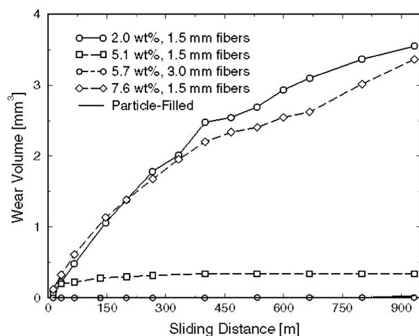
**Figure 2** Specimen volume loss versus sliding distance for an applied load of 4.45 N for all specimens.
