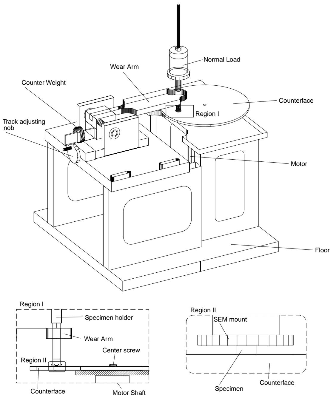
Figure 1 Experimental pin on disc set-up.
