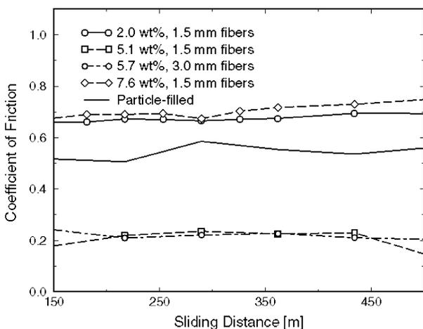
**Figure 10** Coefficient of friction versus sliding distance for an applied load of 22.24 N for all specimens.
