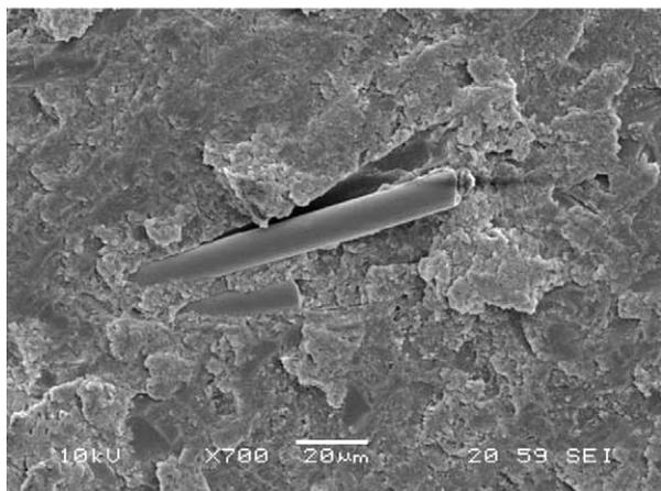
**Figure 5** This SEM of the wear surface of a 2 wt% specimen shows the detachment of the fiber from the surrounding matrix which leads to fiber plucking.
