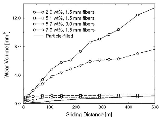
**Figure 4** Specimen volume loss versus sliding distance for an applied load of 22.24 N for all specimens.
