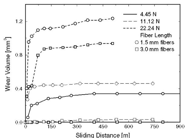
**Figure 8** The effect of the fiber length on the wear volume of the fiber-reinforced bio-composite for all load conditions.
