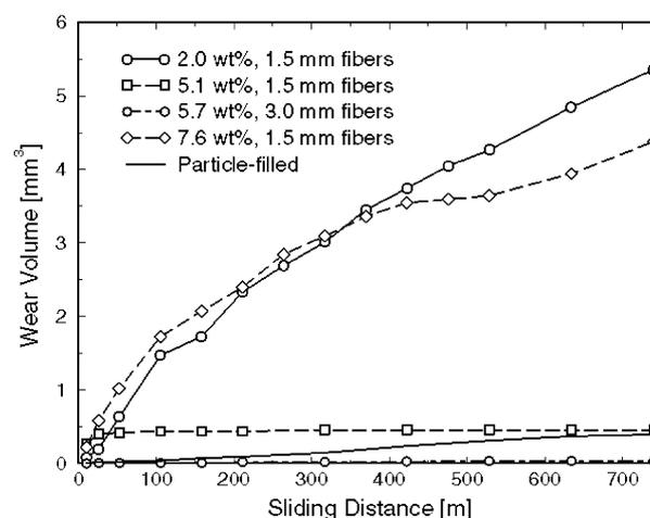
**Figure 3** Specimen volume loss versus sliding distance for an applied load of 11.12 N for all specimens.
