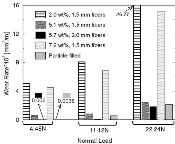
**Figure 9** Average wear rate over the first 500 m of sliding distance for all specimens and all load conditions.
