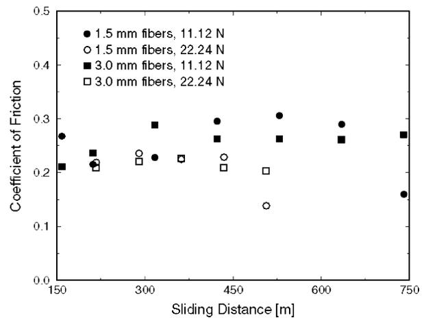
**Figure 11** Coefficient of friction versus sliding distance for different fiber lengths for applied loads of 11.12 and 22.24 N.
