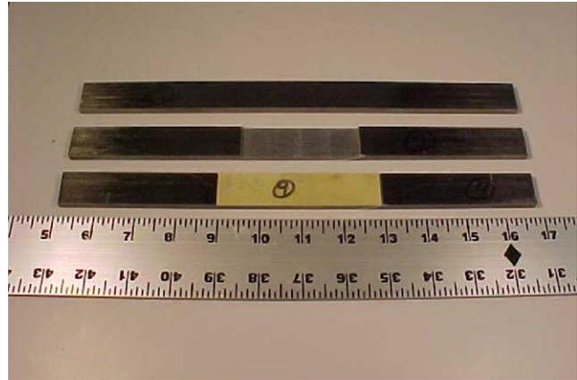
Fig. 3. The manufactured composite beams, before and after machining, and with a repair patch.
