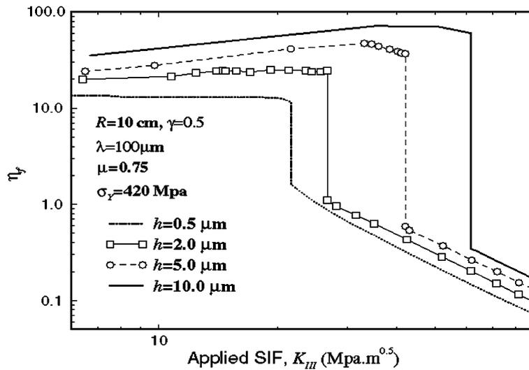
Fig. 11. Variation of the loss factor due to the friction of the mating fracture surfaces,  $\eta_f$  vs. the applied Mode III stress intensity factor,  $K_{III}$  for various average asperities heights.
