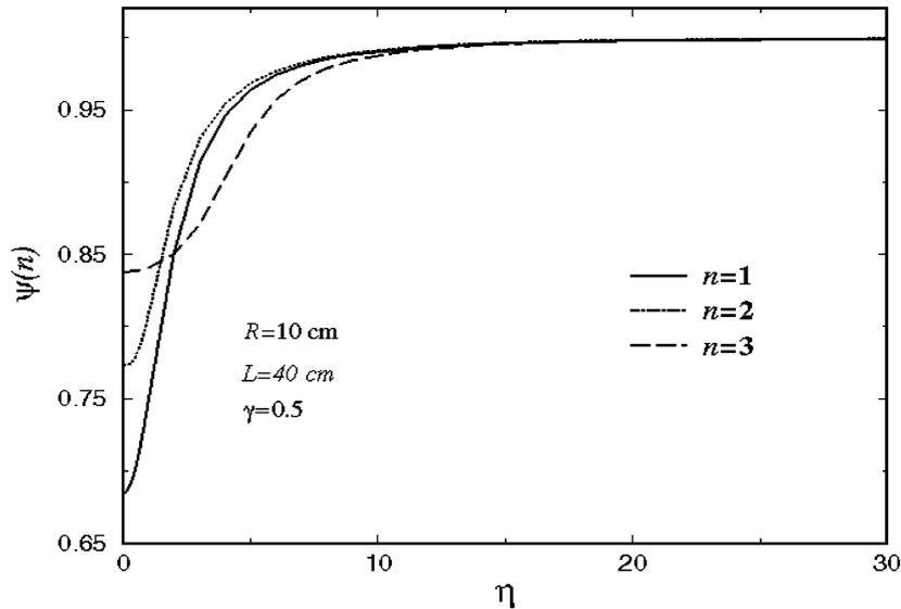
Fig. 14. Variations of the first–third non-dimensionalized peak response frequencies of the shaft with a circumferential crack,  $\gamma = 0.5$  vs. the local loss factor, for a cracked located at the middle of the bar,  $l_1 = l_2$ .
