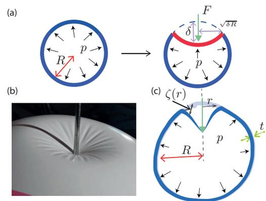
Fig. 1: (Colour online) (a) Schematic illustration of the mirror-buckling of a pressurized shell: an indentation depth  $\delta$  is accommodated by the (energetically cheap) formation of an inverted cap of width  $(\delta R)^{1/2}$ . (b) In reality, an indented pressurized shell wrinkles [16]. (c) Setup and notation for the model calculation of point indentation of a pressurized spherical shell presented here.
