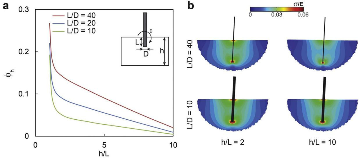
Fig. 3. (a) Saturating characteristic of rotational stiffness of the scales-substrate interaction (b) Comparison of von-Mises stress distribution to show stress concentration for  $h/L = 2$  and 10 for two different values of  $L/D$ . The stress distributions are shown at  $\theta = 0.05$  rad.
