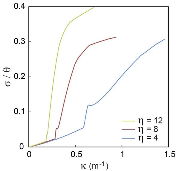
Fig. 5. Normalized deviation of the scale rotation from theoretical prediction versus bending curvature of the substrate,  $\kappa$  for three different values of  $\eta = 4, 8, \text{ and } 12$  for  $N = 48$ .
