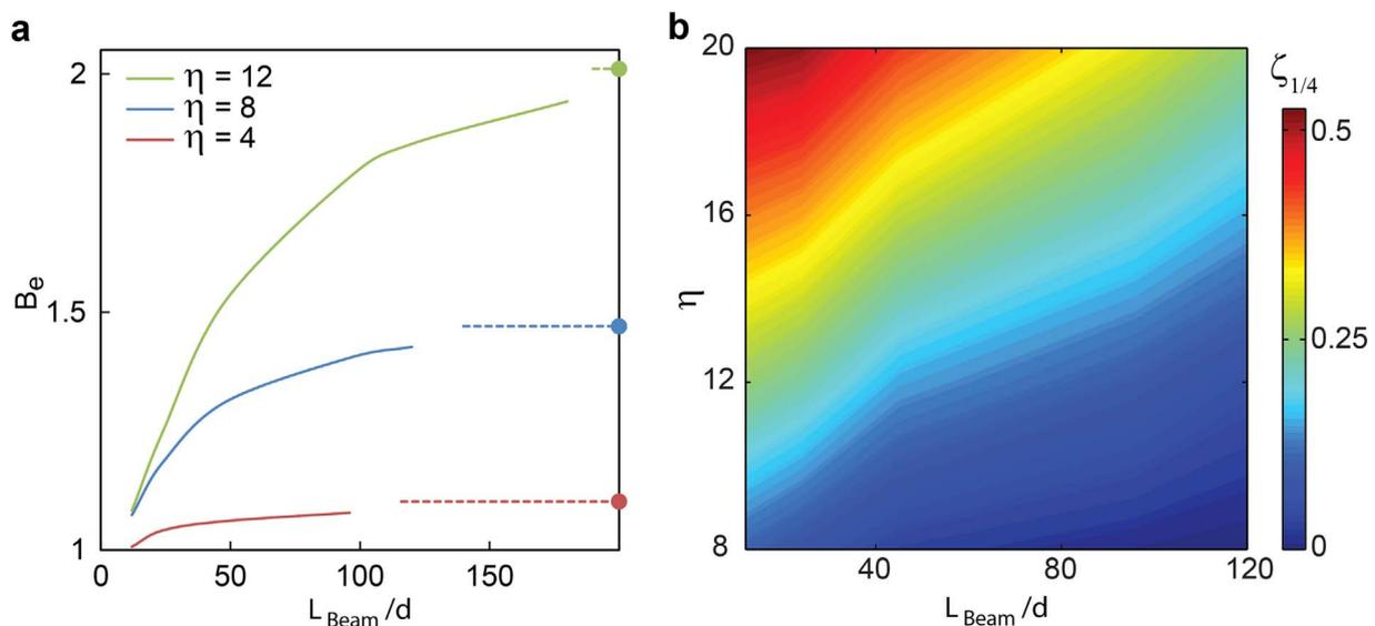
Fig. 6. (a) Variation of the relative rigidity at engagement,  $B_e$ , with the absolute number of scales. The dotted lines show theoretical prediction based on infinity assumption. (b) Relative additional elastic energy density of the biomimetic structure at  $\frac{1}{4}$  the locking curvature spanned over overlap ratio,  $\eta$  and absolute number of scales.
