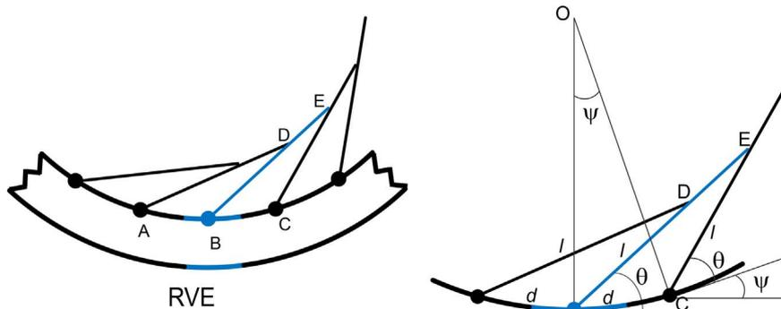
Fig. 2. RVE geometry of the biomimetic structure under bending load. (Adopted from Ghosh et al. APL (2014)).
