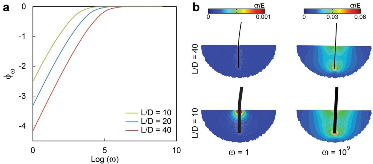
Fig. 4. (a) Saturating characteristic of rotational stiffness of the scales-substrate interaction versus Young's modulus ratio of scale to substrate for  $h/L = 10$ . The figures spans from  $\omega = 1$  (i.e. scale and substrate have materials with same Young's modulus) to  $\omega = 10^9$ . (b) Von-Mises stress distribution shows stress concentration for  $\log(\omega) = 0$  and 9 at  $\theta = 0.05$  rad.
