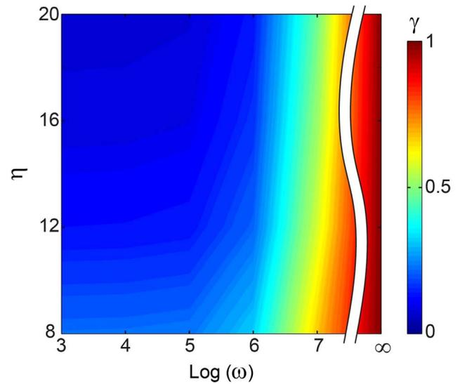
Fig. 7. Variation of the relative rigidity at engagement for the case of non-rigid scale normalized by the rigid assumption results,  $\gamma$ , spanned over overlap ratio,  $\eta$  and stiffness ratio of scale and substrate ratio,  $\eta$  and absolute number of scales.
